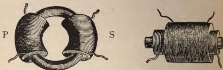
FIGS. 172-173.—Illustrating two types of transformer. The first is the "Faraday ring," a coil of iron wire on which two separate helices are wound. This is the model for the standard repeating coils. The second is an ordinary double wound transformer with "laminated" core, like the common induction coils.
